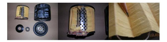
The **Fram** PF7 has the smallest filter area of the four "large" filters measured, smaller even than several "small" filters. The element has cardboard end caps. Only it and the AC/Delco do not use steel element housing. The filter does have a unique base plate design that diffuses oil upon entering the can, perhaps to relieve the stress on the cardboard element.
