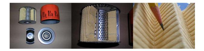
**Mann** filters are made in Germany and sold here by Beck-Arnley, among others. Very sturdy appearance, pleats well-secured against element, nice even pleat pitch. Button bypass, textured media, and the best-fitting gasket of the bunch. Good specs for its small size. At the time of this comparison, the most-expensive filter of the group.
