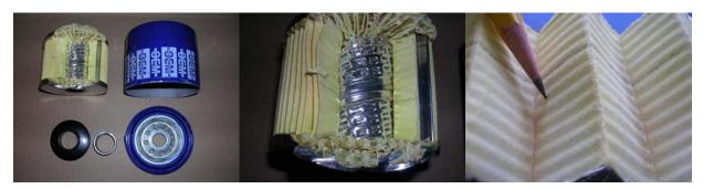
**Purolator** invented the oil filter in 1923. The L20020 has a well-made appearance, although the gasket is easily dislodged. Third place in terms of filter area, but not off by much. Like the Wix, a bypass pressure half that of the Italians, so you may need to change it more frequently. Probably the best value of the lot, as they are available everywhere, though the store may have to order it for you.
